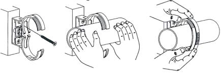
Simply mount CLIC, push pipe in by hand, grips and locks by applying slight pressure. To open: unlock the CLIC latch with screwdriver.
